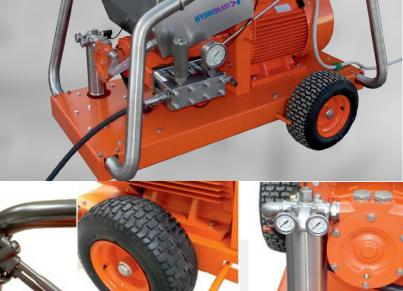
Integrated booster pump & filter system.
