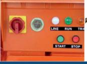
Die cast electrical box with main switch, overload relay & hour meter.
