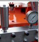
Stainless steel pumphead. Integrated cooling for plunger-seals.
