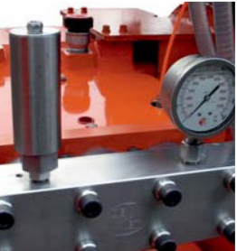
Stainless steel pump-head. Integrated cooling for plunger-seals.
