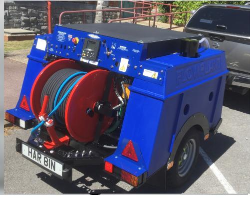
The DTK 3010 trailer drain jetter is perfect for jetting in domestic or light commercial drainage systems. It works at 3000 psi and 10 gpm so it can tackle most drain jetting jobs.
